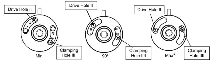
Figure 2: Right Hand Projecting Arm Cam Positions
