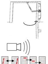
v). Sound the alarm and push the red RELEASE button. There must be no background noise while the alarm is recording
