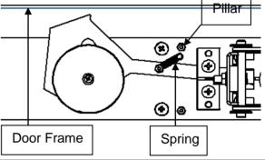
Separate the door closer arm and fit the adjustable arm segment to the door frame using 2 x N°8 \* 1-1/4"
