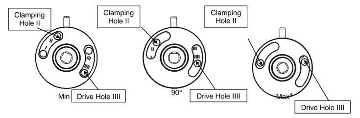
Figure 4: Right Hand Parallel Arm Cam Positions
