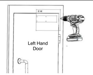
Fit the closer baseplate securely to the door using the  $4\,x$  N°8 \* 1-1/4" screws. Place the free end of the spring over the topmost pillar on the baseplate
