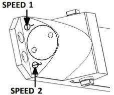
Screw in (clockwise) to slow down, screw out (anti-clockwise) to speed up. Make sure the speed is sufficient to fully close the door
