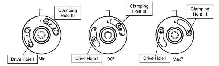
Figure 3: Left Hand Parallel Arm Cam Positions
