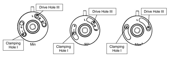
Figure 1: Left Hand Projecting Arm Cam Positions
